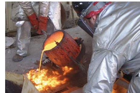
Sand scratch molds filled with iron pour.
