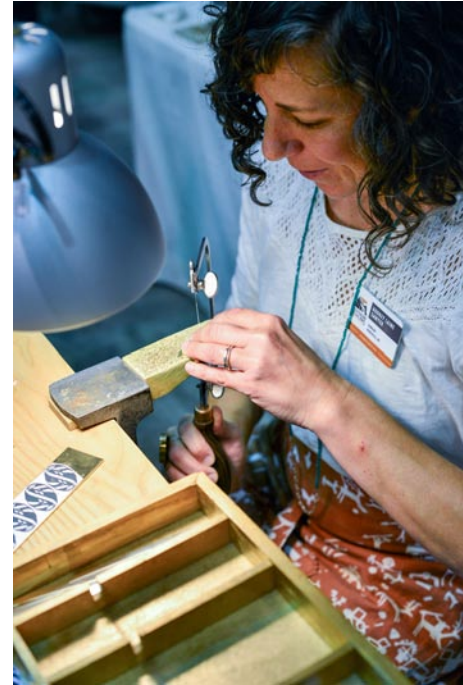
Sawing metal is one of Audrey Laine Sawyer's primary methods to creating her jewelry aesthetic.
